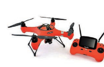
Waterproof drone for collecting red tide samples
